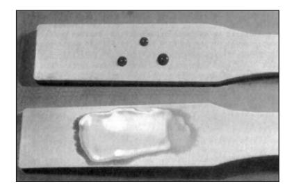
Softening and weakening of the surface occur, leading to the formation of cracks. Liquid adhesive may penetrate into the crack causing further damage. Eventually, the crack may propagate through the entire part and cause failure.
