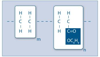
Fig. 4a: Molecular structure of EBA copolymers
