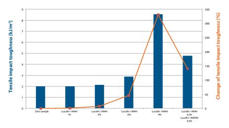
Fig. 12: Improvement of mechanical properties of a PP/EVOH (PP: 86 %, EVOH: 14%) blend by adding Lucofin 1400HN/Lucofin 1494H-tensile impact toughness
