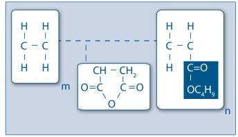
Fig. 4b: Molecular structure of MAH grafted EBA copolymers
