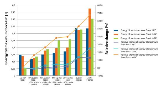
Figure 8: Puncture impact behaviour of LDPE/Lucofin 1400 HN blends- Energy till maximum force Em at various temperatures
