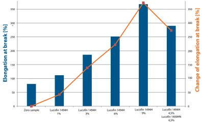
Fig. 13: Improvement of mechanical properties of a LDPE/EVOH (LDPE: 86 %, EVOH: 14%) blend by adding Lucofin 1400HN/Lucofin 1494H elongation at break
