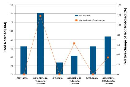
Figure 5: Notched Izod Impact Strength of various PP types compounded with 20 % Lucofin 1400 MN
