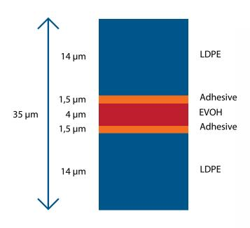
Figure 10: Design of a typical mulitlayered agricultutal film; due to the incompatibility of the constituting polymers not recyclable
