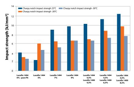
Figure 7: Impact strength of PA modified with Lucofin 1494/Lucofin 1400MN
